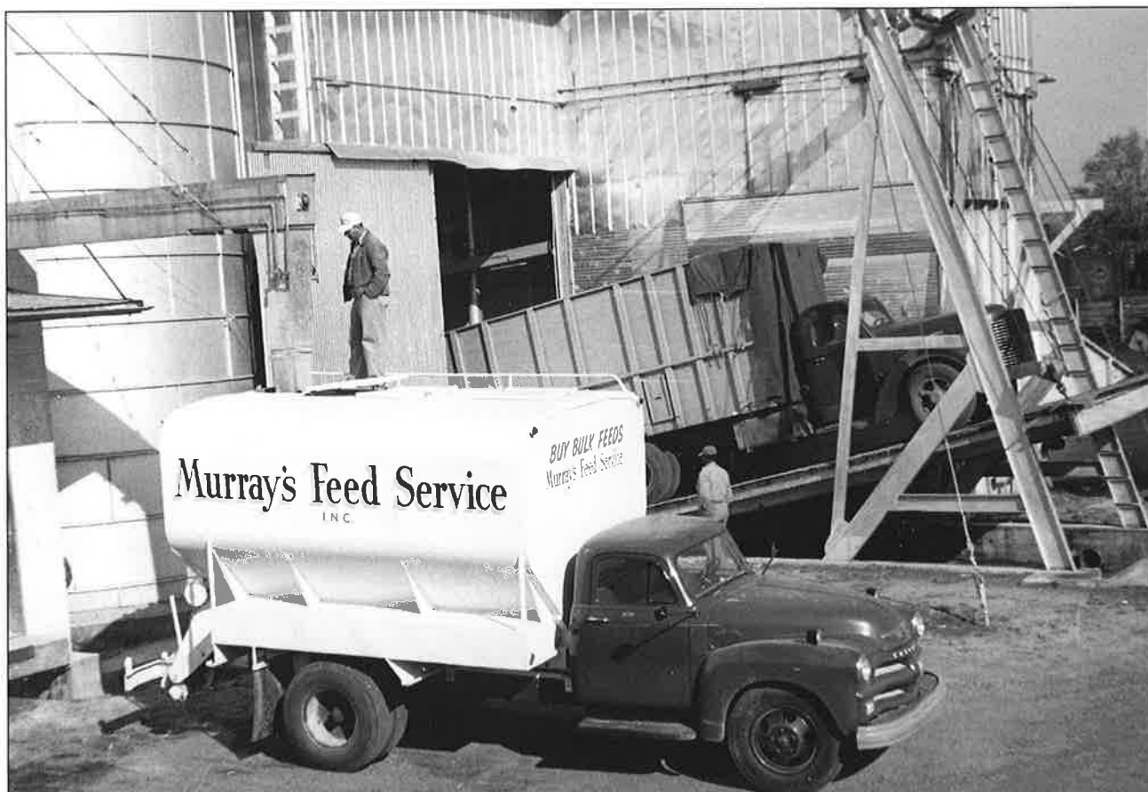
A nine-ton capacity, pneumatic, bulk-feed delivery truck is being loaded with feed at Murray's Feed Service, Inc. mill in Frankford.
